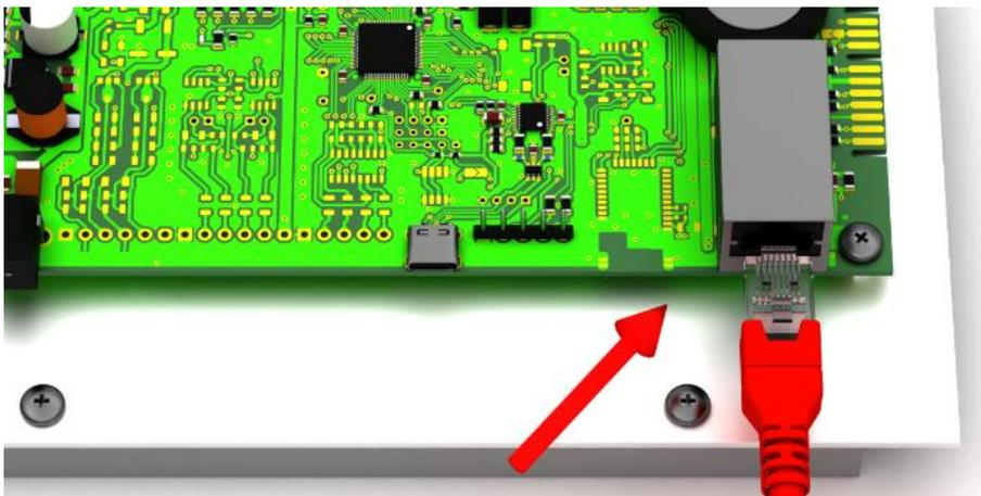
Displays with Ethernet interface are connected with an Ethernet cable cat. 5 or higher. Modern PCs or laptops recognize the cable type automatically.
