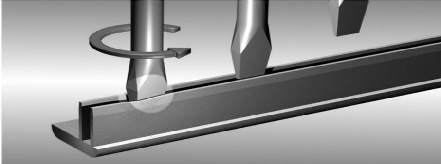
Insert the front pane and the connectors. Spread the connectors slightly with a screwdriver before inserting so that they are stuck firmly in the housing frame. Check that the connectors are fixed so tightly after insertion that they can not be removed without tools (lever tools).
